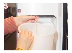
Place in the refrigerator with the tube in the container and press Ok. When prompted, remove the container and clean the milk tube.
