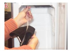
Clean the milk tube and hose with clean wet towel. Place milk back in refrigerator. Press Exit to finish cleaning.
