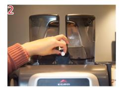
Place an Egro Coffee Machine Cleaning Tablet in the chute on top of the machine.
